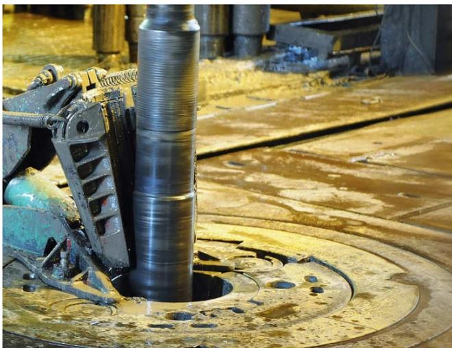
Figure 9 Drill pipe tooljoint passing through rotary table
