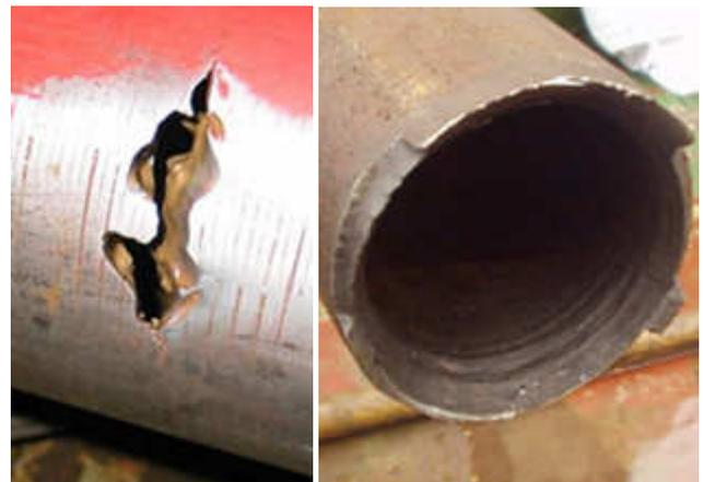
Figure 1 Examples of drill pipe failures. Washout in 5” drill pipe (left) and twist-off in 3 ½” drill pipe (right). If a wash-out is not detected through monitoring drilling parameters the result is normally a parted string down hole.
