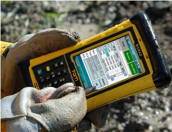
Figure 5 Ruggedized handheld computer with RFID reader. (Also available in ATEX zone 1).
